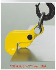
The THK horizontal plate clamps share the same basic design features as the CH range of clamps but have a reversed tooth jaw design. This safety feature is designed for use with thin sheets which may have a tendency to deflect or sag or flex.
