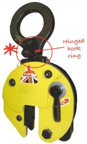
The CY plate clamps with hinged hook rings can be used for the safe handling of plate at various angles. It can lift plate from the horizontal and put it down in the vertical. The hinged hook ring ensures adequate gripping pressure in every position, but the load capacity reduces. See the diagram below showing the load / force capacities.
