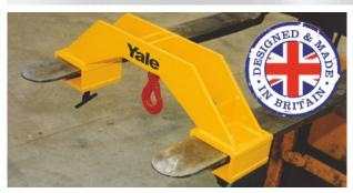
The FLTH tine hook is designed to convert your forklift truck into a crane. This is done by simply sliding the FLTH over the tines of your forklift truck. The FLTH is fastened to the tines by tightening the two threaded bars underneath each tine. The unit is supplied a standard with a swivel safety hook.
