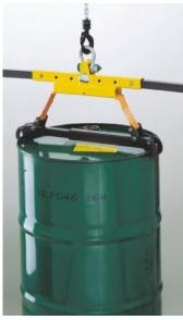
**The DA drum grab** is designed for the vertical transportation of steel drums. The jaws grab under the lip of the drum with its form-fitting connection.
