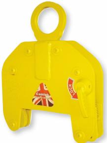
The TJC twin jaw vertical plate clamps have been specifically designed for lifting materials with low minimum weight, but large thickness. The main difference between the TJC and the CZ (which is our standard vertical plate clamp) is that the TJC has a unique twin moving jaw arrangement
