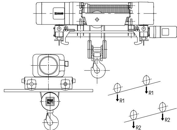
**DRT DOUBLE GIRDER TROLLEYS FOR DRH ELECTRIC WIRE ROPE HOISTS – TRANSVERSAL 2 FALL (2/1) AND 4 FALL (4/1) VERSIONS**
