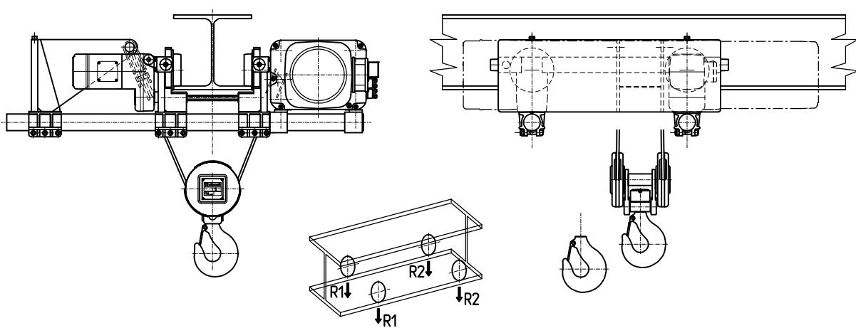
**DRT DOUBLE GIRDER TROLLEYS FOR DRH STANDING/SUSPENDED ELECTRIC ROPE HOISTS - 2 FALL (2/1) AND 4 FALL (4/1) VERSIONS**
