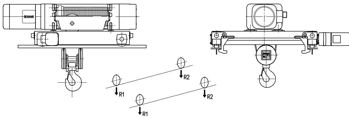
**DRT DOUBLE GIRDER TROLLEYS FOR DRH ELECTRIC WIRE ROPE HOISTS – TRANSVERSAL 2 FALL (2/1) AND 4 FALL (4/1) VERSIONS**
