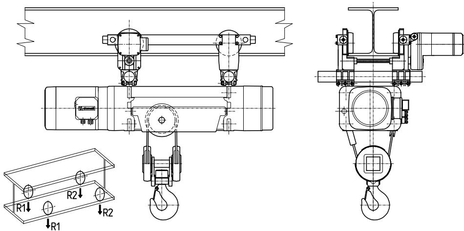
**DST/R MONORAIL TROLLEYS FOR DRH ELECTRIC WIRE ROPE HOISTS – 2 (2/1) FALL VERSION**
