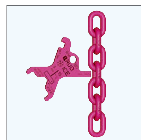
Testing for pitch elongation caused by wear of nominal diameter
