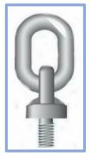
The eye of a collar eyebolt is too small to accept a hook so a shackle is always needed as the first item of any connection. However BS 4278 does offer a third option and that is the eyebolt with link.
