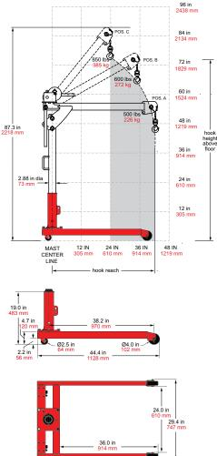
**IMPORTANT:** Crane DOES NOT rotate in base when assembled in 5BR5 wheel base.
