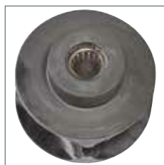
Load chain sheave with needle bearing
