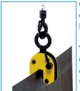
Generally the initial grip of cam types comes from a spring operated by a lever which the user flips over into the locked position after positioning the clamp on the plate.
