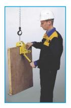
However there are non-marking clamps designed to handle plates of harder material or which have delicate surfaces where indentations from the clamp teeth would be unacceptable.
