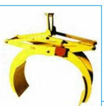
proportion to the load lifted. The self-weight of the clamp tends to close it and therefore provides the initial grip.
