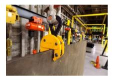
Clamps are the ideal tool for handling loads safely by overhead crane or hoist.
