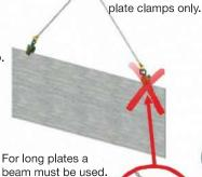
For long plates a beam must be used. Do not use endless chain slings.
