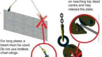
When the clamp is wrongly positioned it will reposition itself on reaching top dead
