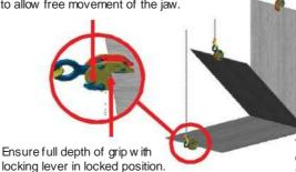
Lifting sling must be vertical for all positions.
