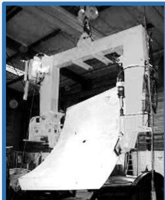
The clamp can also incorporate a mechanism for orientating the load so, for example, the facing panel of a building can be transported and stored flat but lifted and turned to the vertical and presented to the building for fixing.
