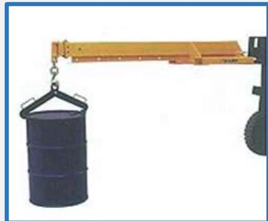
This method of handling is much safer than balancing an unstable load over the forks and provides the ability to rotate and position the load much more safely and precisely. (Continued)
