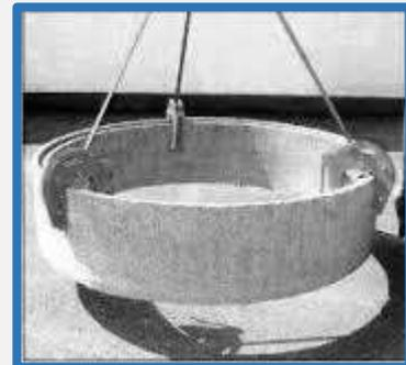
Clamps offer a method of connecting to the load so that it may be presented tight up to a neighbouring component without trapping the lifting equipment.
