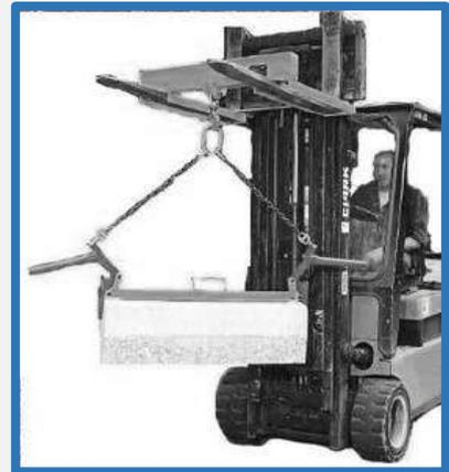
Some clamps are designed specifically as permanent attachments to a hydraulic arm on a road vehicle or site truck.
