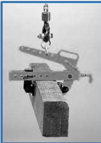
Whether it is [manhole segments](#), kerbstones, safety barriers, [pipes](#) or any other pre-cast concrete products, there are clamps designed to lift and position them.
