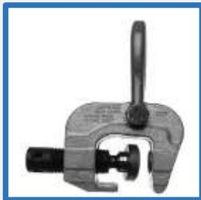
The simplest designs utilise a screw thread which is manually tightened to grip the load. They are particularly useful for applications where the clamp is to be left in place between a series of handling operations.
