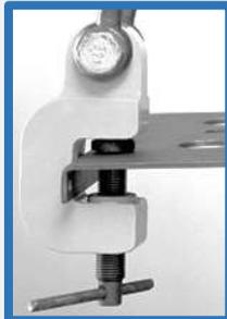
The clamping force can be produced in a variety of ways. The simplest is by means of a screw thread.
