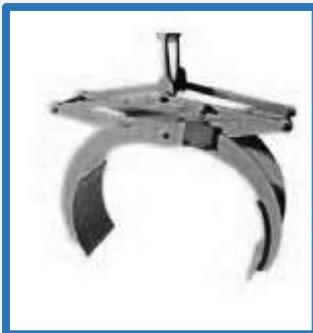
proportion to the load lifted. The self-weight of the clamp tends to close it and therefore provides the initial grip.
