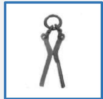
They have to be locked open in order to release the load and this can be by means of either a manual lever or by an automatic latch.
