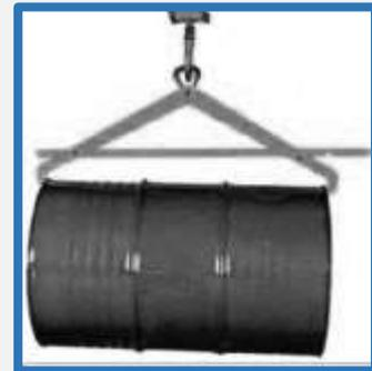
In addition to lifting drums vertically, there are clamps which lift drums in the horizontal position.
