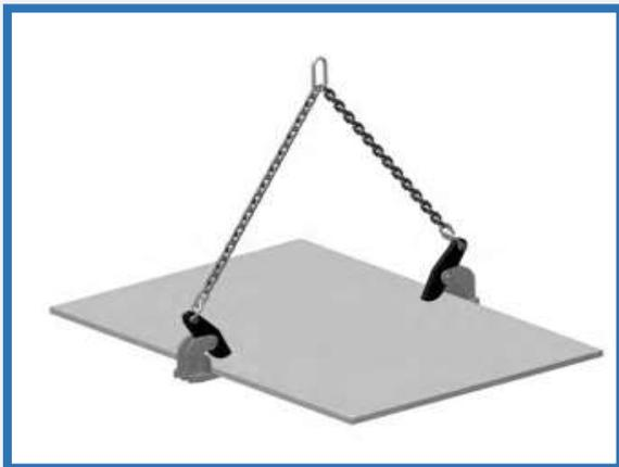
As the name implies, horizontal plate clamps only handle plate laid flat. They are therefore always used in pairs, one either side of the plate, in conjunction with a two leg sling.
