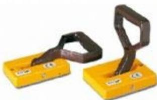
The THM manual magnetic claw is used for transporting steel sheets horizontally and vertically, lifting plates from racks, pulling steel sheets out of shelving, as well as transporting flat pieces of magnetisable steel.
