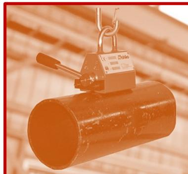
Therefore when lifting a particular type of load for the first time, it is good practice to check that an adequate adhesive force is achieved.
