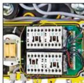
Increased operating safety through 42V control voltage
