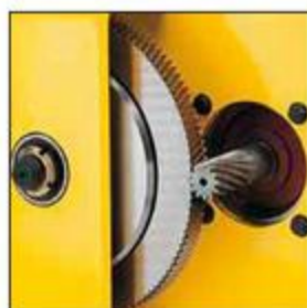
Gearbox with slip clutch
