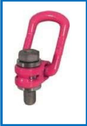
**VLBG Load Ring** will turn 360°, adjustable in pull direction. Load ring foldable, full WLL in any load direction, surface pink powder coated. The max. lengths of the RUD - bolts are adjusted in such a way that if a hex-head-shaped nut (DIN EN ISO 7042) is used, assemblies of material thickness of approximately 8 \*M (for M8 - M30) and 5 \*M for (M36 - M48) can be realised respectively.
